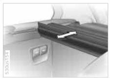
When the cover is pulled out, it can be opened behind the rear-seat backrest to gain access to the cargo area from the rear seats during a trip, for example.
