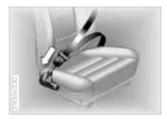
The safety belt tensioner responds to collisions by tightening the belts to ensure that occupants remain firmly positioned in their seats. A gas-pressure system retracts the buckle assembly to tension the shoulder and lap belts within fractions of a second. This reduces the tendency to slide under the lap belt.
