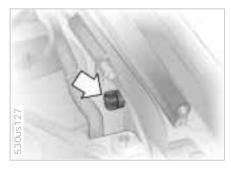
5 Then connect the negative terminals. Attach the cable to either the support vehicle's negative battery terminal (-), or to a suitable ground on its engine or bodywork. Then connect the other end of the cable to a ground on the engine or on the bodywork of the vehicle that is to be started. There is a special nut for this on the left side panel of your BMW. Refer to the arrow in the illustration.
