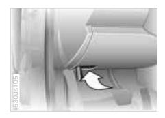
The Onboard Diagnostic (OBD) interface socket is located on the left of the driver's side at the bottom of the instrument panel and under a cover.
