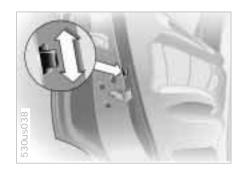
Slide the safety lever on the rear doors downward:
