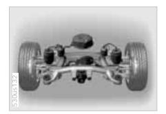
The level control system for the rear axle maintains constant ground clearance of your vehicle, even when carrying a load.
