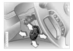
The steering wheel can be moved in any of four directions. Adjust the wheel by moving the control lever in the desired direction.
