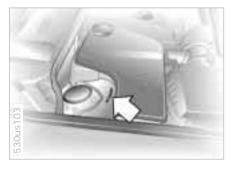
In the engine compartment, stamped on the right-hand strut dome (arrow) and on the upper edge of the instrument panel on the left-hand side.
